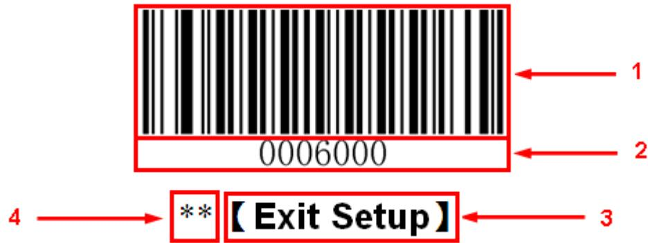
The figure above is an example that shows you the programming barcode and command for the **Exit Setup** function:
